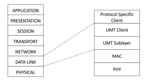
UMT Exists in the Data Link Layer of the OSI Model
