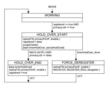
Figure 9-411—Trunk protection process operating on the ONU
