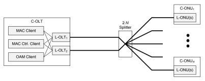
Figure 9-18—Trunk protection with redundant L-OLT
