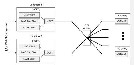
Figure 9-29—Trunk protection with redundant C-OLT
