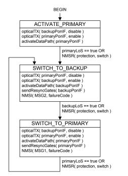
Figure 9-<u>310</u>—Trunk protection process operating on the OLT
