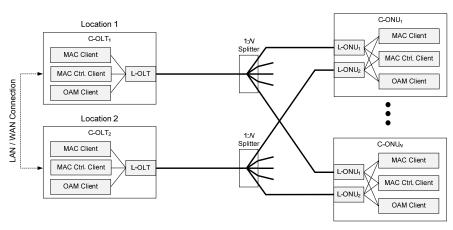
Figure 9-613—Tree protection with redundant C-OLT
