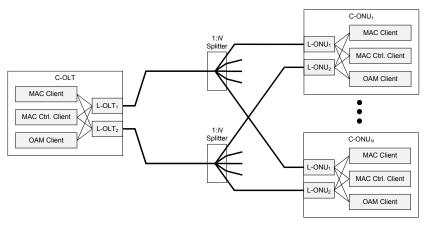
Figure 9-512—Tree protection with redundant L-OLT
