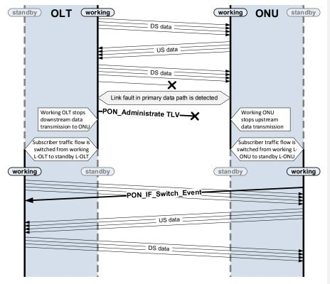
Figure 9-845—An example of tree protection switching: link failure detected by working OLT and working C-ONU
