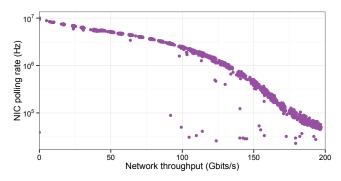
Figure 10: As more requests are handled, the NIC polling rate decreases. The resulting queueing delay can be bounded by distributing request-handling across multiple comm-cores.
