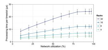
Figure 12: Path selection routes traffic from 16 racks of 32 endpoints in <12  $\mu$ s. Consequently, 10 pathsel-cores would output a routing every <1.2  $\mu$ s, fast enough to support 10 Gbits/s endpoint links. Error bars show one standard deviation above and below the mean.
