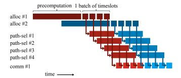
Figure 6: Multicore allocation: (1) allocation cores assign packets to timeslots, (2) path selection cores assign paths, and (3) communication cores send allocations to endpoints.
