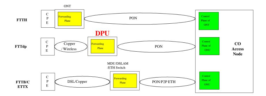
• Control planes of remote nodes are moved to the aggregation OLT, while remote nodes implements forwarding plane.
