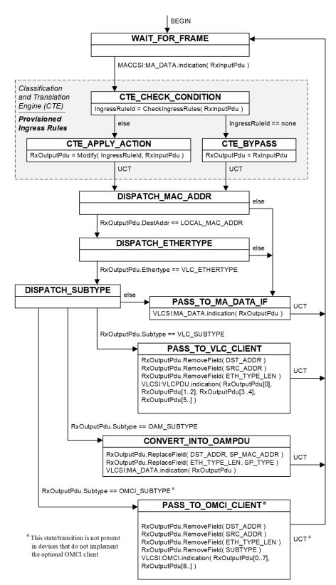
Figure Error! No text of specified style in document.-1—Receive process state diagram
