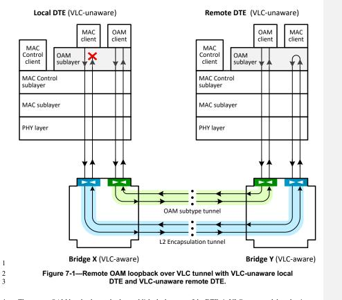
4 The remote OAM loopback can also be established when one of the DTEs is VLC-aware and the other is not.
