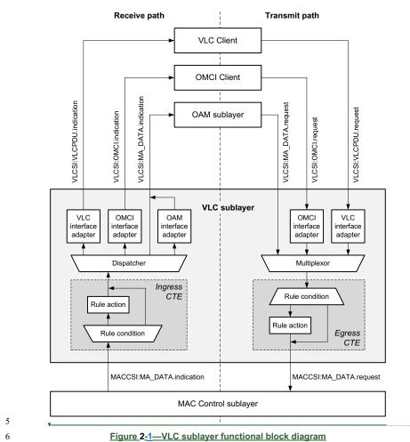
The VLC sublayer includes a set of interface adapters and the Classification and Translation Engine (CTE). Together these functional blocks convert xPDUs into VLCPDUs and vice versa. The CTE behavior is
