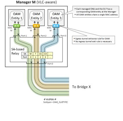
Manager M to manage multiple ONUs while minimizing the resources required to do so. The example described in 8A.5.1 requires one MAC instance, and one MAC address, on Manager M for each ONU that is under management. This is because the recipient VLC sublayer relies on the source MAC address to distinguish between tunnels. In other words, Manager M relies on the source MAC address on ingress VLCPDUs to determine which OAM entity should receive the VLCPDU.
