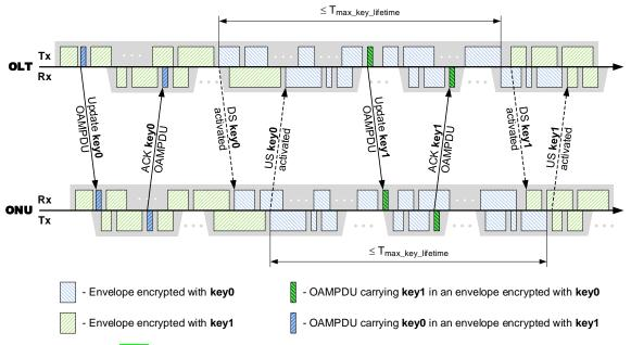
Figure 11-x – Key update and subsequent key activation time diagram
