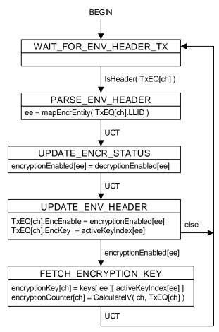
Figure 11-xxxxx -- ONU encryption key activation process state diagram
