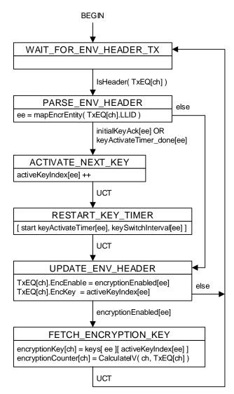
Figure 11-xxx -- OLT encryption key activation process state diagram
