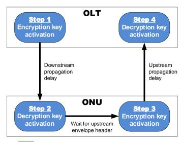
Figure 11-xx – Four steps comprising the key activation procedure
