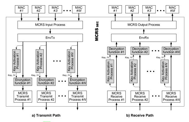
Figure 11-1 – Location of encryption/decryption function within MCRS<sub>SEC</sub>
