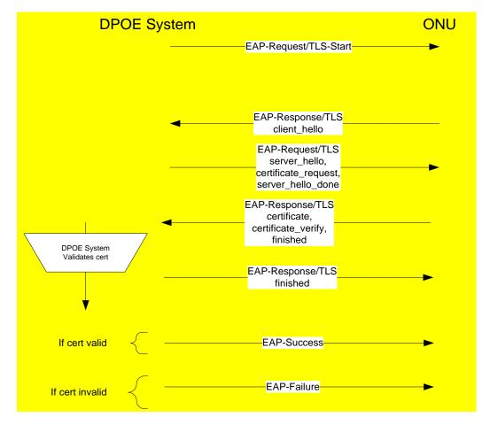
Figure 1 - EAP-TLS Message Sequence
