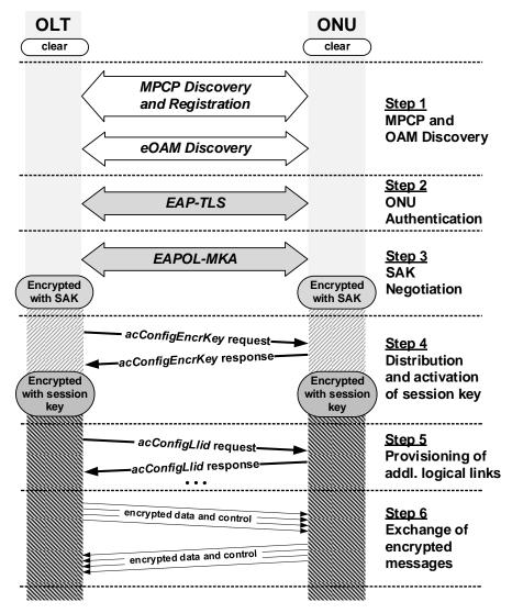
Figure 15-1 - Sequence of steps to establish secure ONU operation
