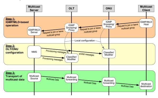
Figure 7-20—Steps establishing multicast operation in EPON
