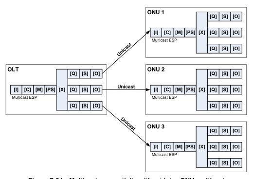
Figure 7-24—Multicast connectivity without inter-ONU multicast
