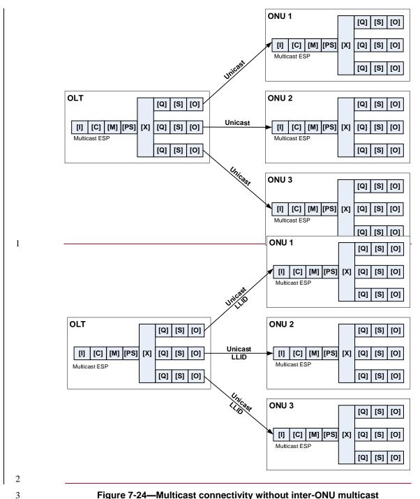
Figure 7-24—Multicast connectivity without inter-ONU multicast
