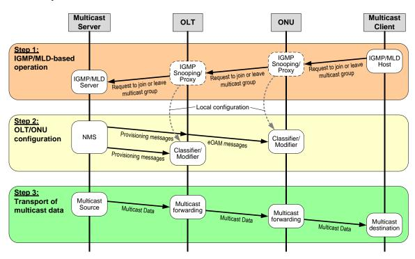
Figure 7-20—Steps establishing multicast operation in EPON
