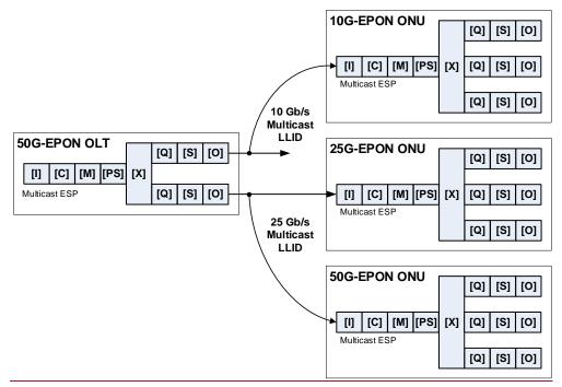
Figure 7-23—Multicast ESP in 1/10G-EPON OLT at the OLT to support 10G-EPON and 25/50G-EPON ONUs
