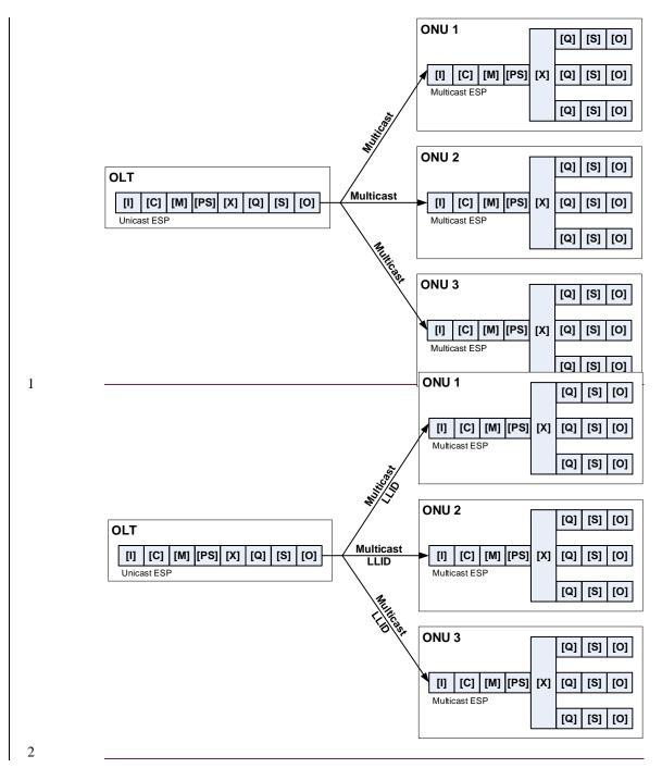
Figure 7-22—Multicast configuration using unicast ESP in the OLT and multicast ESPs in the ONUs
