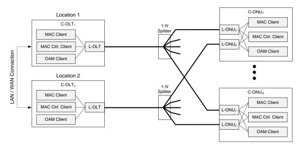
Figure 9-8—Tree protection with redundant C-OLT
