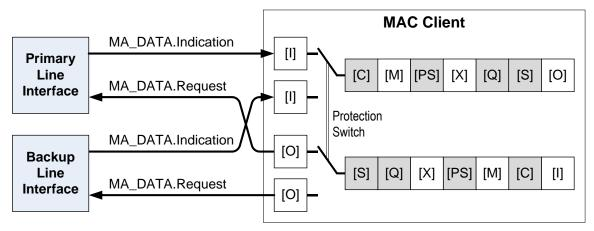
Figure 9-1—Line device protection architecture
