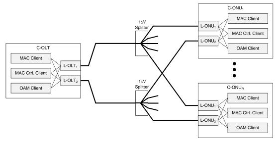
Figure 9-7—Tree protection with redundant L-OLT
