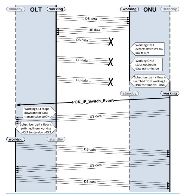
Figure 9-12—An example of tree protection switching: downstream link failure detected by working ONU
