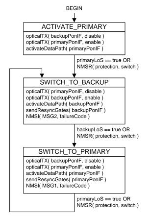
Figure 9-5—Trunk protection process operating on the OLT
