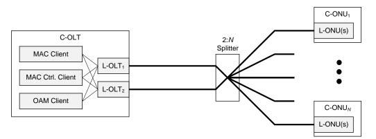
Figure 9-3—Trunk protection with redundant L-OLT
