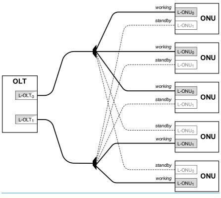
Figure 9 -x—L-OLT ports connected to working and standby L-ONUs
