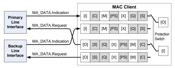
Figure 9-2—Client device protection architecture
