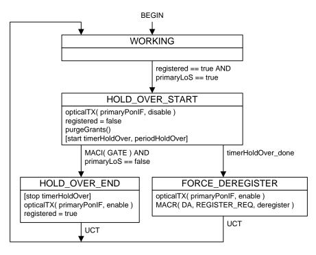
Figure 9-6—Trunk protection process operating on the ONU
