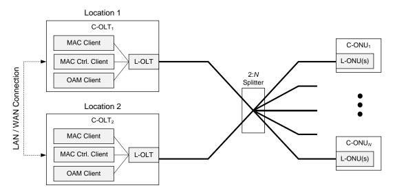
Figure 9-4—Trunk protection with redundant C-OLT
