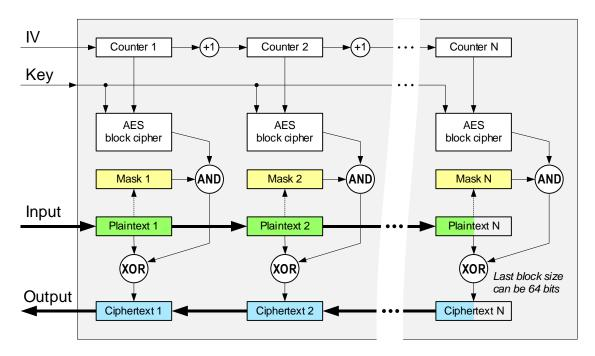
Figure 11-xx1 – Block diagram of the encryption process
