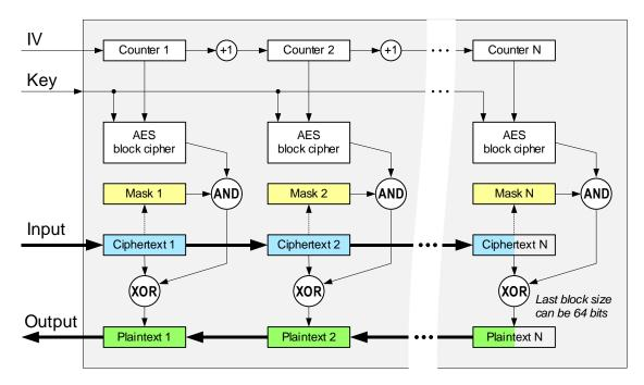
Figure 11-xx2 - Block diagram of the decryption process
