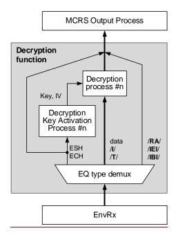
Figure 11-x3 – Decryption function block diagram.
