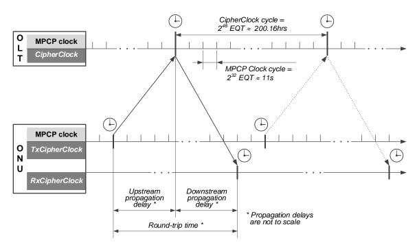
Figure 11-xx4 - Relationship of OLT's CipherClock and ONU's TxCipherClock and RxCipherClock
